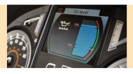
Oil level check on CF and XF Driver Information Panel now shows either current level or last oil level readings with date and mileage information
